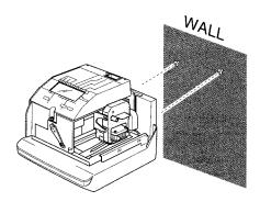
Unlock the key and remove the cover. And then hang it on the wall.
