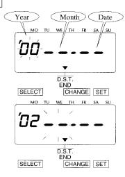
Press the <u>SELECT</u> button and position the ▼ over the "D.S.T. END".
