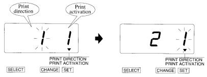
Press the SELECT button and position the ▼ over at the "PRINT DIRECTION; PRINT ACTIVATION".
