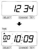
In case of the example, press the CHANGE button to set at "34". And then press the SET button. At that moment, the ▲ mark indicates the "TIME".
