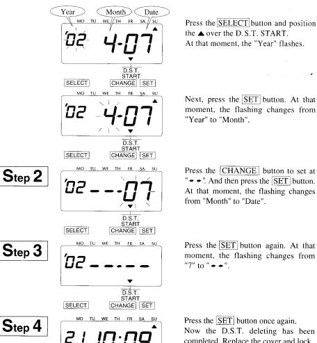
Press the SET button once again. Now the D.S.T. deleting has been completed. Replace the cover and lock.
