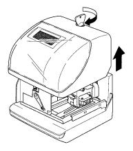
Unlock the key and remove the cover.
