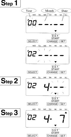
Press the **SELECT** button and position the ▼ over the "D.S.T.START". At that moment the "Year" flashes. (The flashing means it can be changed)
