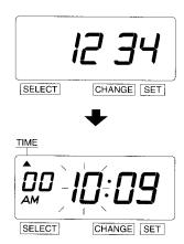
In case of the example, press the CHANGE button to set at "34". And then press the SET button.
