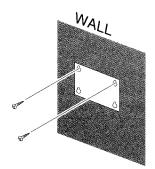
Install the supplied wall-mount screws into a wall by using the template.
