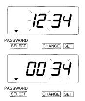
Press the SELECT button and position the ▲ mark at the "PASSWORD".
